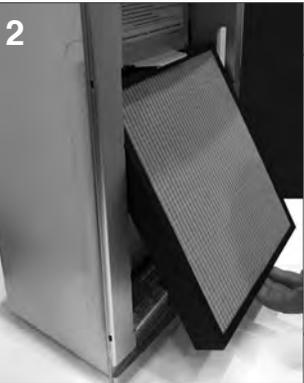
Remove the 5 stage pre-filter, the pre-filter should be cleaned monthly by using a small vacuum cleaner and replaced every 6-12 months. (2)
