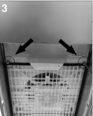
To replace the main filter; using a screwdriver, remove the 2 screws, holding the main filter in place. Remove the main filter, discard the main filter using the filter bag of the new main filter. (3)
